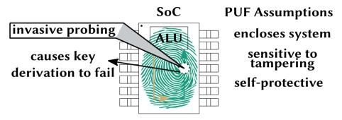
tamper-evident PUF = protection from probing attacks
