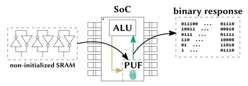
key <u>derivation</u> from response instead of key storage! advantages: delayering and optical analysis cannot reveal key disadvantages: noisy response necessitates error-correction
