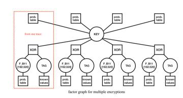
The outputs of this step are the probability tables of candidates for fragments of K, Note that when attacking the unmasked version, we could use 16-bit fragments, because where the probability has been updated by belief propagation.
