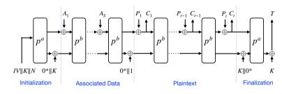
Attack strategy: Our setting is a profiled fixed-length known plaintext attack. In the profiling stage, the attacker knows the plaintexts P, associated data A, keys K, nonces N, ciphertexts C, and tags T, along with recorded power traces. In the attack stage, only the tags T and recorded power traces are needed to recover the secret key K.
