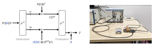
During the attack phase, we recorded traces of up to 10 encryptions, each with the same key K, but varying plaintext P. For the key enumeration step, we limited the search to enumerating up to 100 000 candidate keys when evaluating the success rate.
