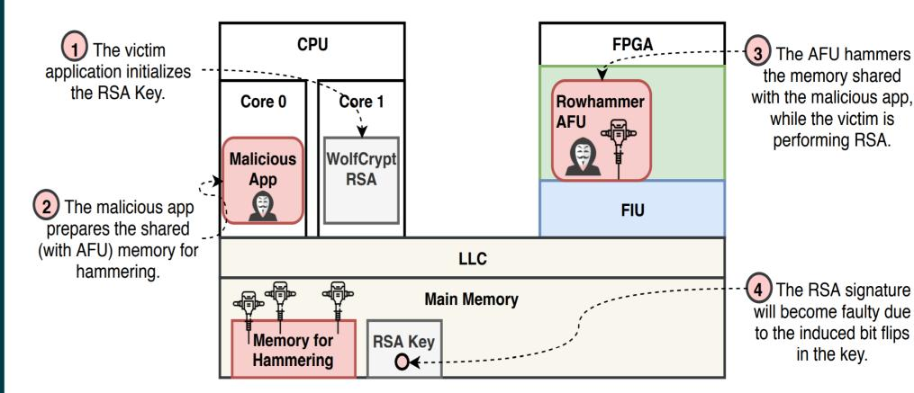
We constructed a **fault injection attack against the RSA signing function in WolfSSL** [2], outlined in the figure above. When using JackHammer instead of a conventional CPU Rowhammer, **a key can be recovered an average of 17% faster**. With some typical defenses against Rowhammer exploits in place, JackHammer is **over three times more likely to cause a fault** than the same attack with CPU Rowhammer.
