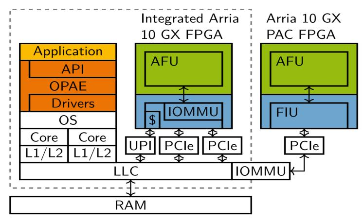
We show a **cache covert channel between FPGA and CPU** and **JackHammer**, which is a Rowhammer attack from FPGA against a host's main memory. It performs **twice as fast** as conventional CPU Rowhammer and causes **four times as many faults**.
