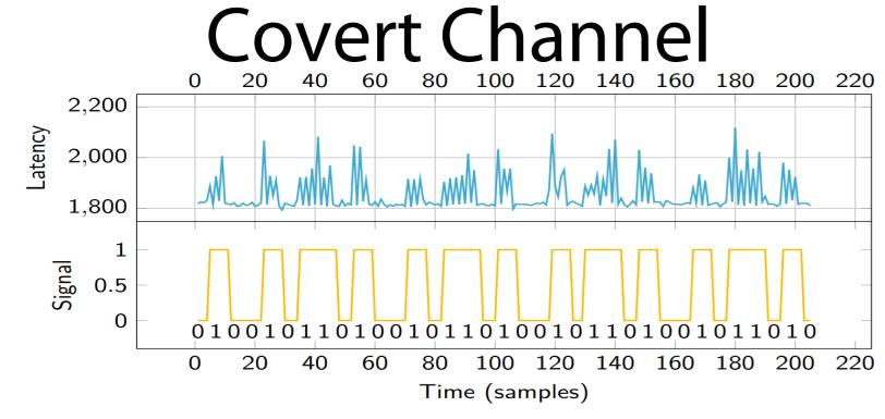
We constructed a covert channel with the FPGA as the sender and a cooperative CPU program as receiver. The **FPGA sends** binary messages by writing to a cache line when transmitting a One and staying quiet otherwise. The receiver continuously probes the cache set to detect access latency fluctuations to receive the messages. While using heavily redundant encoding, we still achieve a throughput of 94.98 kBit/s.
